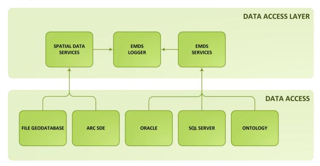
**Figure 3.** Data Services Tier. Data storage functionality is hidden behind services and objects that are accessed by the Business Logic Tier (Figure 4).
