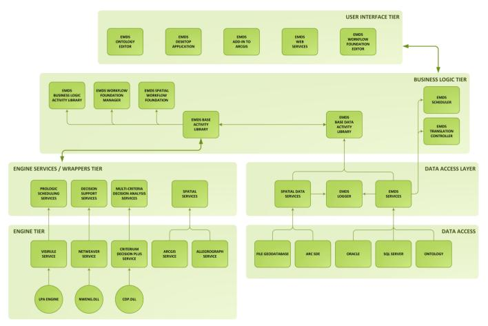
Figure 1. Overview of the EMDS 5 service-oriented architecture.
