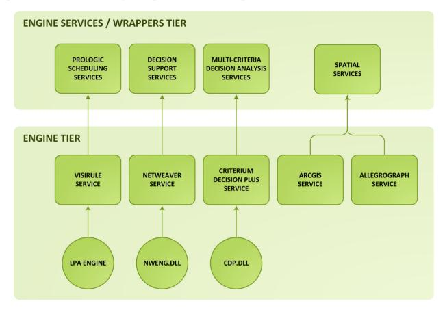
**Figure 2.** Engine Services Tier. NET wrappers provide the interface to each engine in this tier.
